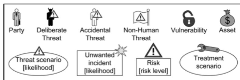
Figure 2.9. Basic building blocks of the CORAS diagrams taken from (Dahl, Hogganvik, and Stølen, 2007)
