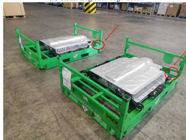
(b) Edge nodes mounted on containers
