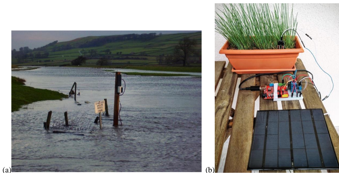
Figure 2.1. (a) A GridStix node taken from [55]. (b) A prototype of hydric stress monitoring system.
