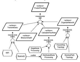
Figure 1 Goal/Operationalization Variability View of GridStix
