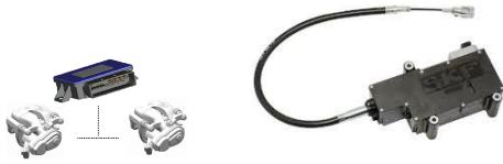
Figure 7: The Electric Parking Brake system main design alternatives ( PullerCable and ElectricActuator variants are required)
